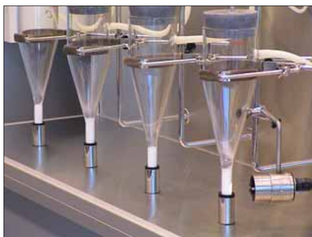
Fig.1 The fluidizing chambers and the NIR-probe
